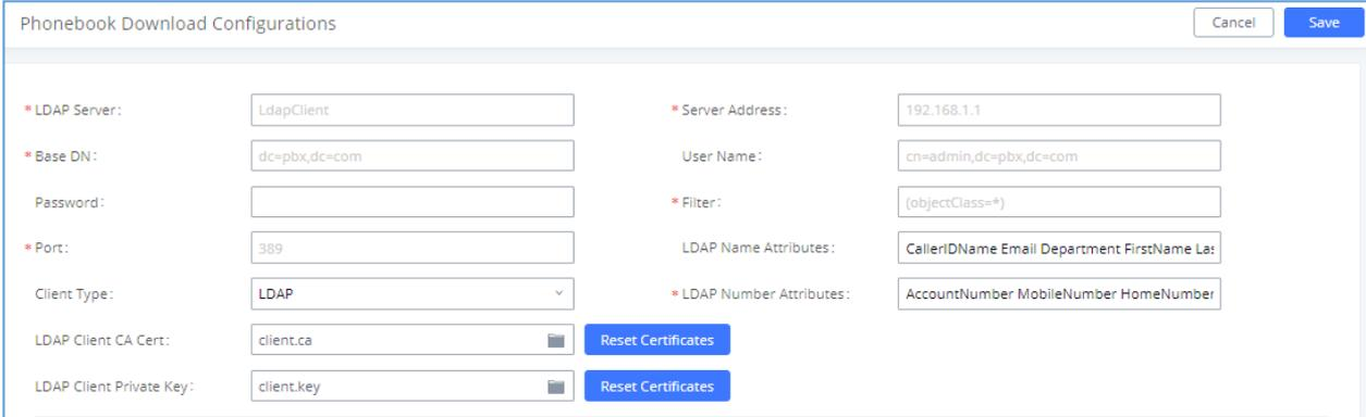
Figure 10: LDAP Client Configuration
