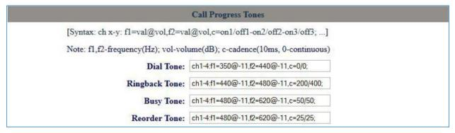
Figure 10: Configure FXO Port on the GXW410X: Call Progress Tones
