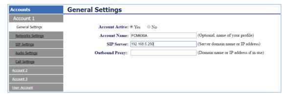
Figure 5: Configure FXO Port on GXW410X: General Settings
