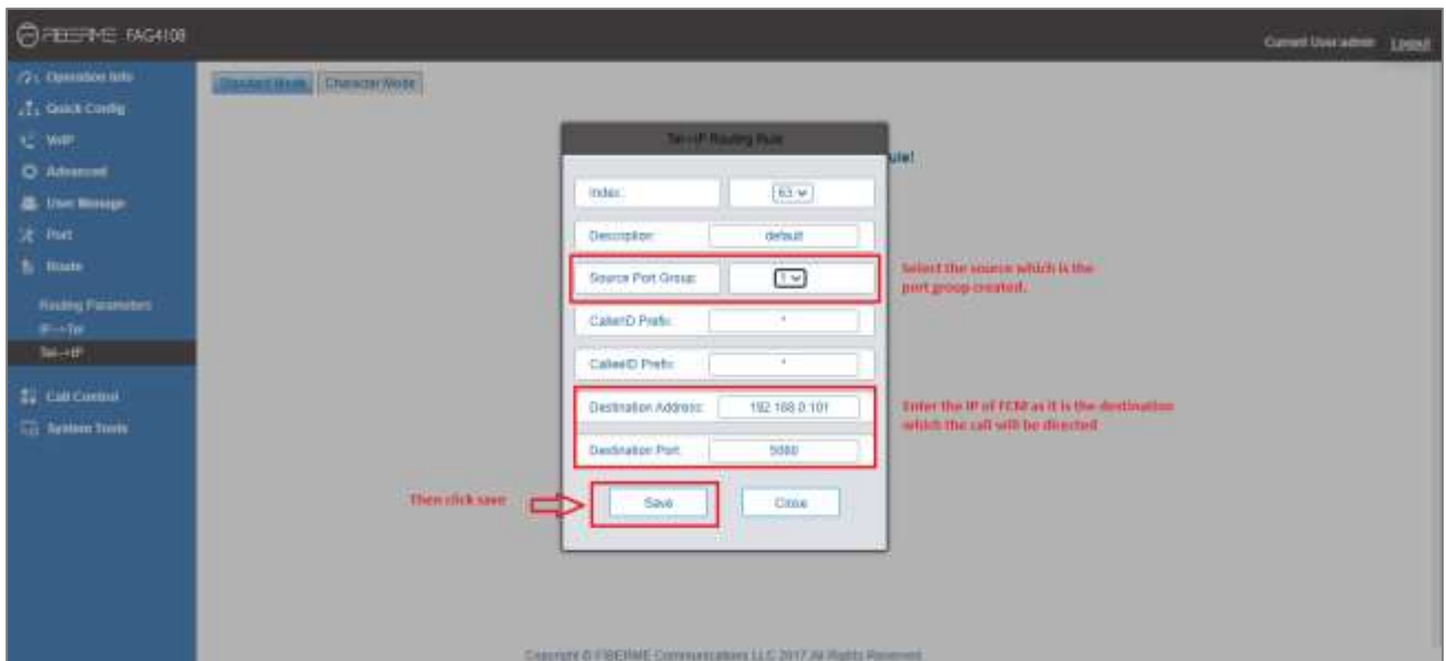
Figure 22: Configure TEL->IP Route
