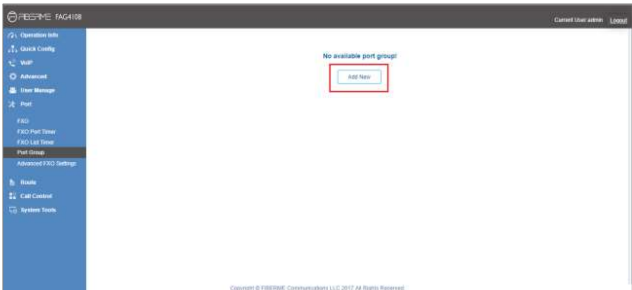
Figure 16: Create Port Group on FAG4108
