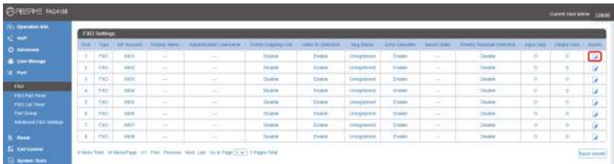
Figure 7: Configure FXO Port on FAG410X: Modify Port
